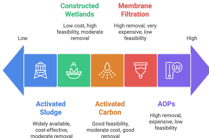
Figure 2. Comparative assessment of wastewater treatment technologies for emerging contaminant removal in Indonesia. Five approaches are evaluated by removal efficiency, cost-effectiveness, and implementation feasibility. Constructed wetlands and activated carbon offer promising options for tropical, decentralized contexts.
